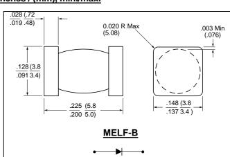
Note: The cathode side is marked with a dark colored band on one side of the diode body.
